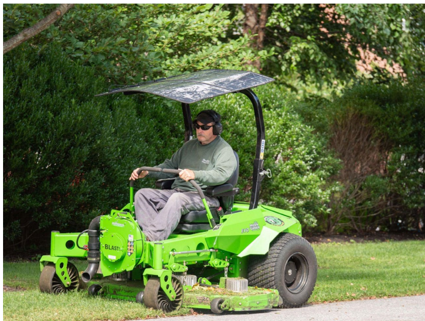
Groundskeeper using electric lawn mower with solar canopy (Source: The Bowdoin Orient )
